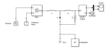
This configuration models a third-order low-pass Butterworth filter with a cutoff frequency of 1 rad/ns, or about 0.159 GHz. The high-frequency mixing product is in the stopband of the filter. The low-frequency product is in the passband.
