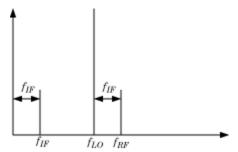
The preceding figure illustrates frequency conversion. A signal modulated on the carrier  $f_{RF}$  mixes with a local oscillator at  $f_{LO}$ . The operation downconverts  $f_{RF}$  to  $f_{IF} = f_{RF} - f_{LO}$ . The upper mixing product  $f_{RF} + f_{LO}$  is not modeled.
