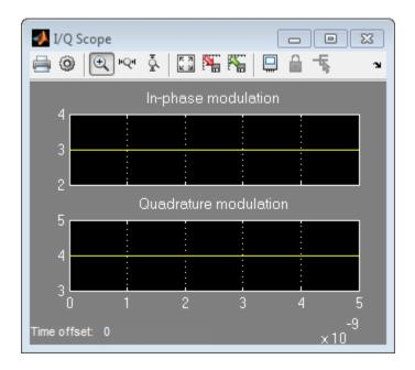
The 1-GHz carrier itself does not appear in the output. The results correspond to the real and imaginary parts of the Complex modulation at the input of the system. They also correspond to the In-phase modulation and Quadrature modulation blocks in "Simulate a Passband Signal in Simulink Software" on page 1-6.
