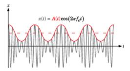
The signal consists of a time-varying modulating signal on a high-frequency carrier. In many RF applications, the frequency of the modulating signal A(t) is much less than the frequency of the carrier,  $f_c$ .
