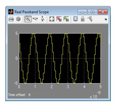
The Real Passband Scope displays the same output as the example in the previous section, "Simulate a Passband Signal in Simulink Software" on page 1-6. The signal has a magnitude of 5 and a phase shift consistent with the specified in-phase and quadrature amplitudes.
